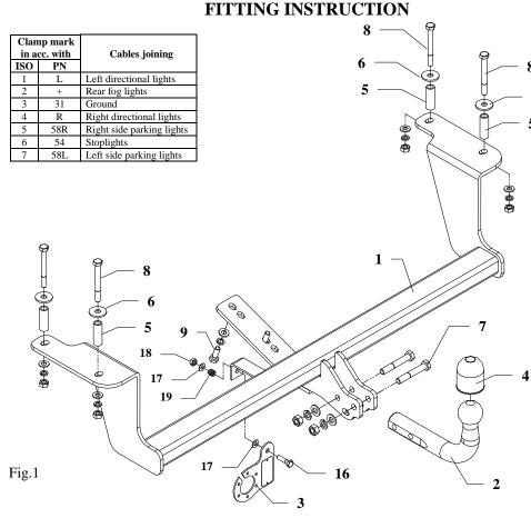
This towing hitch is designed to assembly in following car: **SUZUKI IGNIS II, 3/5 doors, 2/4WD,** produced since 09.2003 till 2008 (in Hungary), catalogue no. **W19** and is prepared to tow trailers max total weight **800** kg and max vertical load **50** kg.
